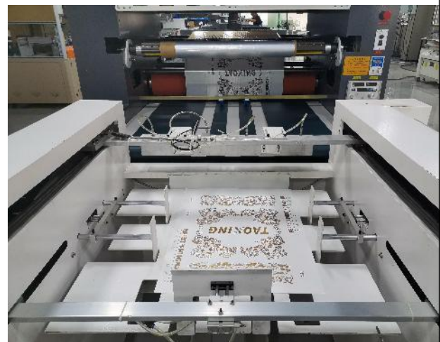
Automatic material receiving machine
